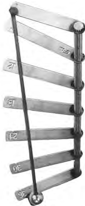
UPPER LEVEL RADIAL ARM GAUGE TREE WITH FLOAT
